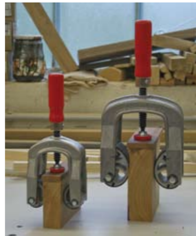
Anleimen von Massivkanten Glueing of massive edges
